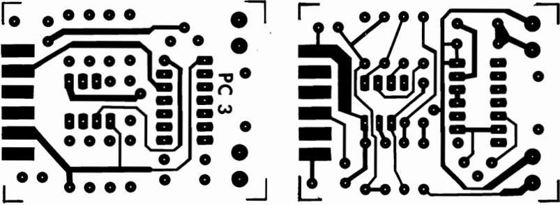
Figure 3.6 PC Board Layout for Circuit 2
