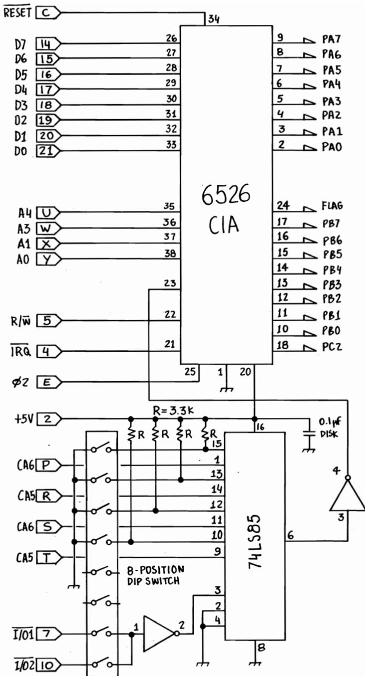
and 57087 inclusive (\$DEOO-\$DEFF). I/O block 2 ranges between 57088 and 57343 inclusive (\$DFOO-\$DFFF). Two signals, I/O1 and I/O2, available at the expansion port, become active low when the corresponding I/O block is addressed.
