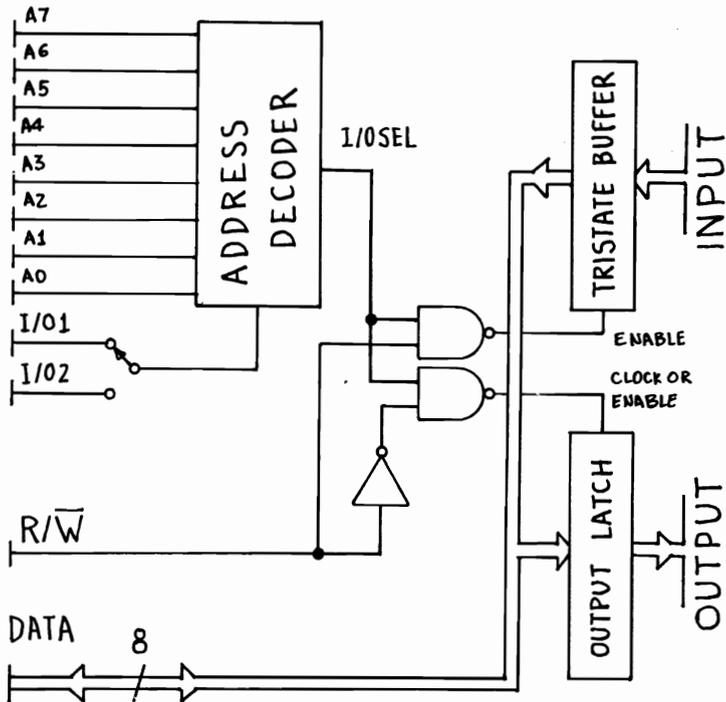
Figure 1.2. I/O Port Block Diagram
