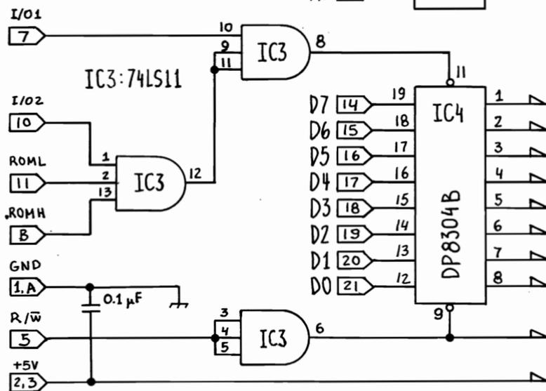
nal. It is enabled only when external access is requested (I/O1, I/O2, ROML or ROMH signals active) so there are no conflicts when accessing locations internal to the 64.
