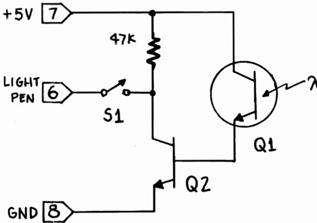
Figure 7.1. Light Pen Schematic
