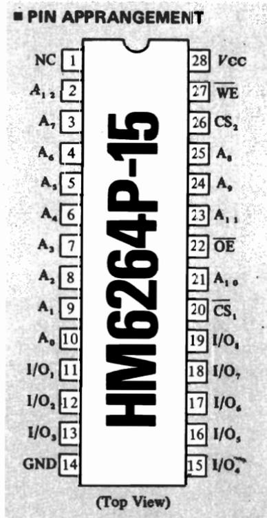
8192-word x 8-bit High Speed Static CMOS RAM
