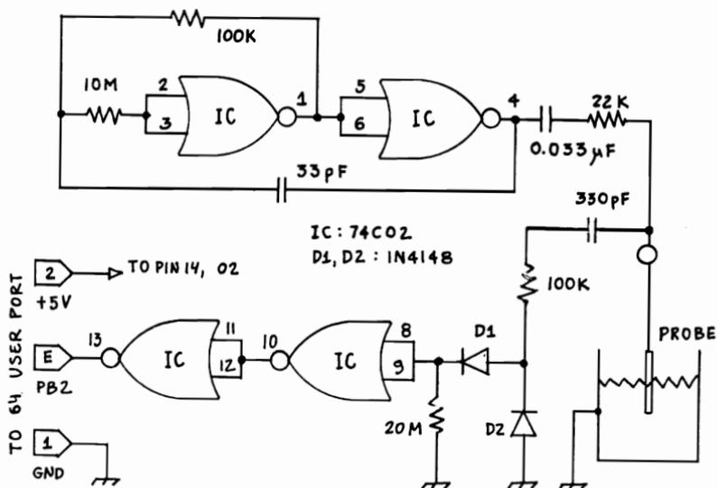
If the container is the liquid if not conductive (for example the basement mentioned above), the probe must have two separate conductors (one of which connects to the circuit ground). In some cases, a phono plug will work fine as the probe. In others, two parallel strips can be etched on a piece of circuit board and used as the probe.
