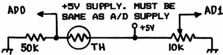
Figure 28.5 Resistance Measuring Circuit
