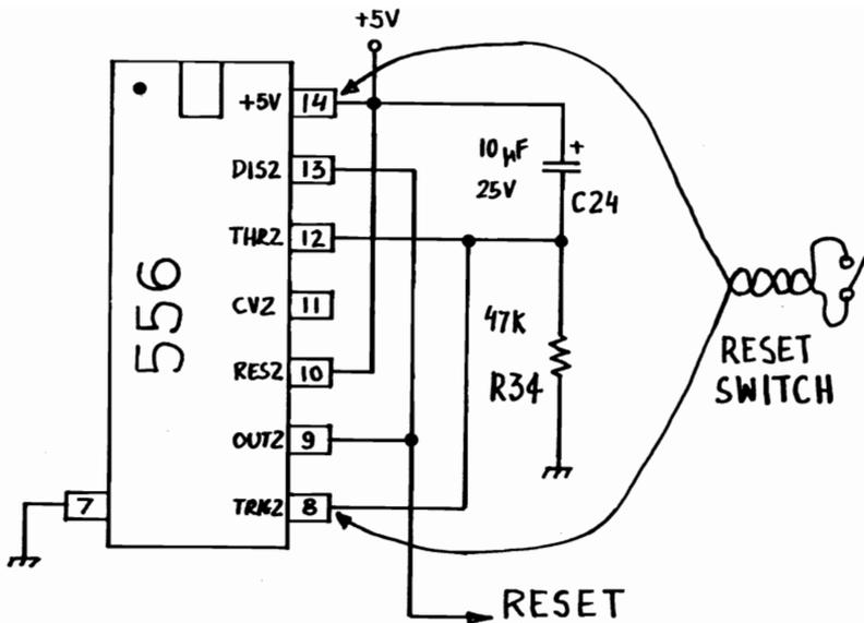
Figure 6.1 Reset Circuit of Later Model 64. The RESET Switch is Added Between Pins 14 and 8
