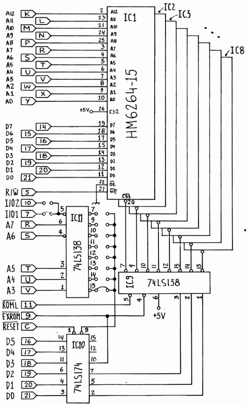
paging, at least for the hardware portion of it. A good page size for the 64 is 8K. We can stack our pages in the address space starting at 32768 (\$8000). This particular area is designed for operation with external ROM, for adding game cartridges or the extended BASIC. Thus, there are provisions in the 64 to switch its own RAM out of this space when external memory is used. The external memory signals its presence by grounding a pin in the expansion port labeled EXROM.
