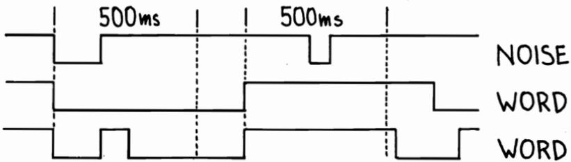
capacitor, C2, the output does not present any jitter for the duration of the sound. A sound, however, is not a word. We define a word as a sound that lasts more than 500 ms. This way, almost all noises are rejected because they normally last less than 500 ms. On the other hand, all words are longer than that, especially if pronounced fully and clearly.
