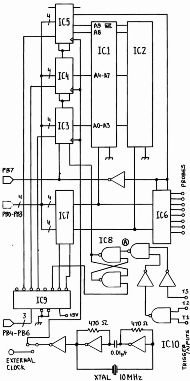
Figure 34.1 Block Diagram of the Logic Analyzer
