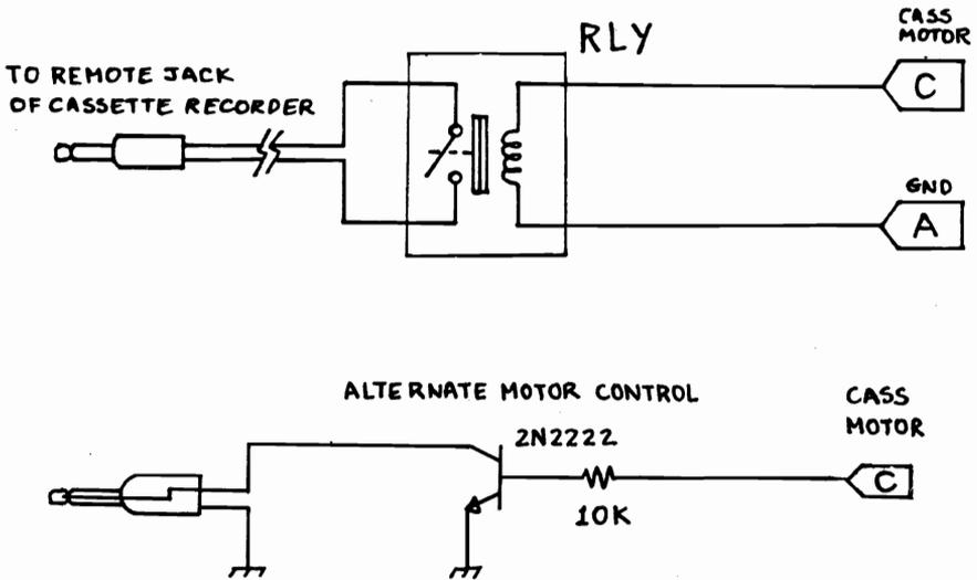
Figure 3.7. Cassette Motor Control Circuits
