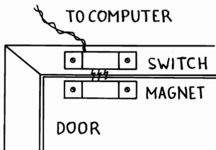
Figure 36.1 Placement of Magnetic Switch on Door
