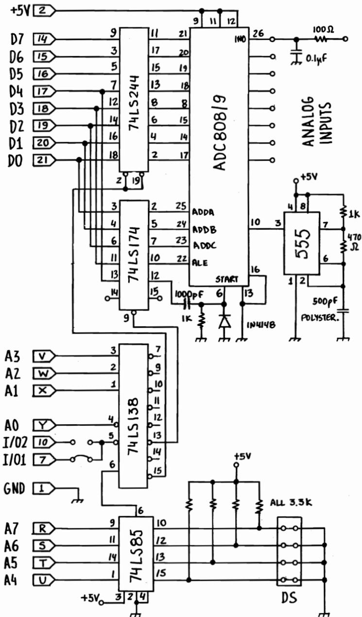
Figure 28.2 Schematic of the 8-Channel, 8-Bit A/D Converter
