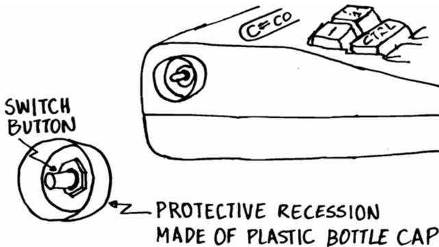
Figure 6.3. Construction Detail of the Reset Switch
