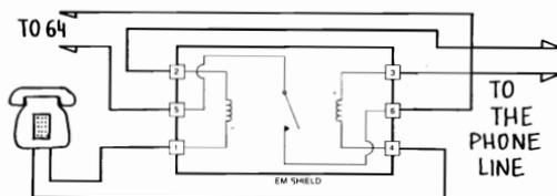
The line sense relay can also be used to count the rotary dial pulses and to recover the number dialed out, either for recordkeeping purposes or just to find out who is calling whom and when.
