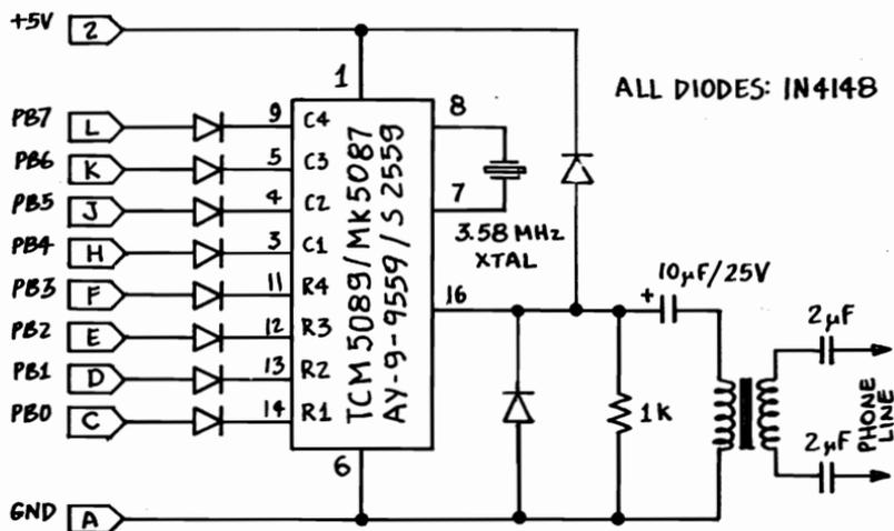
tion. A good quality transformer is needed here for reliable operation. The important specification is flat frequency response in the DTMF frequencies (600 to 1700 Hz).
