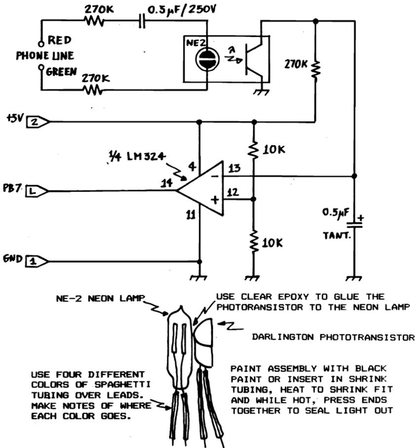
picked up by a Darlington phototransistor. The resulting signal is amplified by an op-amp and presented to the user port as a logical '0' or '1'. The use of the neon lamp gives excellent noise immunity because the lamp does not fire at voltages less than 70 volts. Thus line noises, clicks, etc. do not give false readings. In addition, it offers perfect isolation of the phone lines since no electrical connection is made between your circuit and the line.
