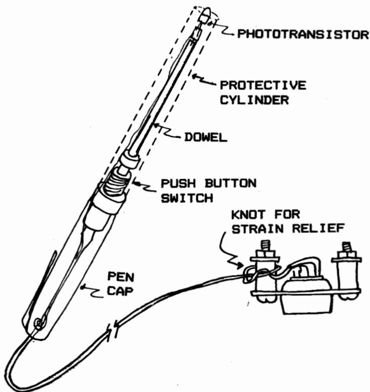
Figure 7.2. Construction Detail of a Push-to-Activate Light Pen
