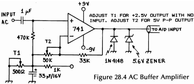
Figure 28.4 AC Buffer Amplifier
