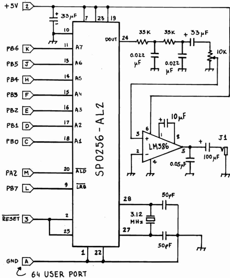
and spoken through an external speaker. When the talking is finished, LRQ goes low signifying the synthesizer is ready for another allophone.
