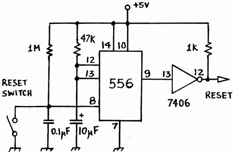
Figure 6.2 Reset Circuit of Earlier Model 64. The RESET Switch is Added Between pins 8 and 7
