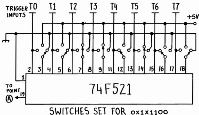
Figure 34.2 Eight Channel Triggering Circuit
