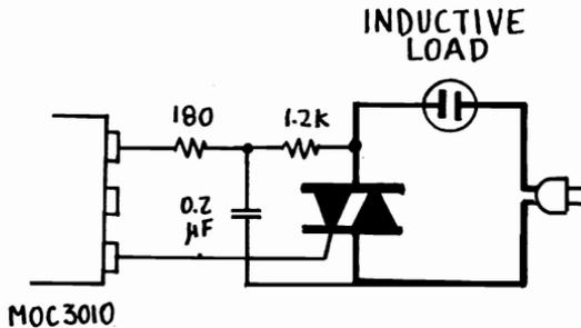
are shown, one for resistive loads (lights, ovens etc.) and one for inductive loads (anything that contains a motor: fans, refrigerators, etc.).
