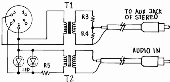
Figure 2.4 Transformer Coupled Audio Connections
