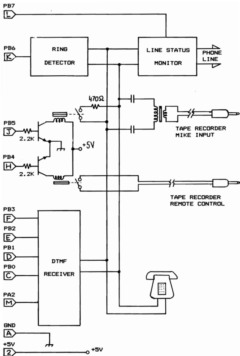
Figure 21.1 Block Diagram of DTMF Receiving Setup
