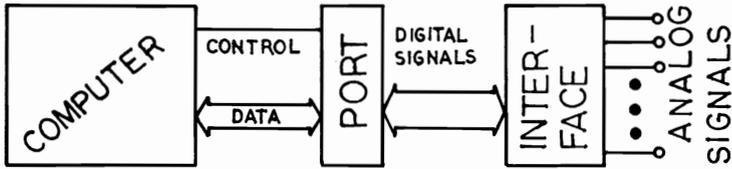
Figure 1.1. Interfacing Block Diagram
