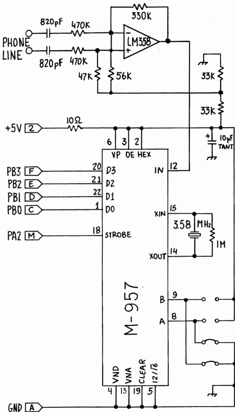
output is "1". The data output of the receiver is connected to bits PBO-PB3 of the USER PORT, while the STROBE output is connected to PA2.
