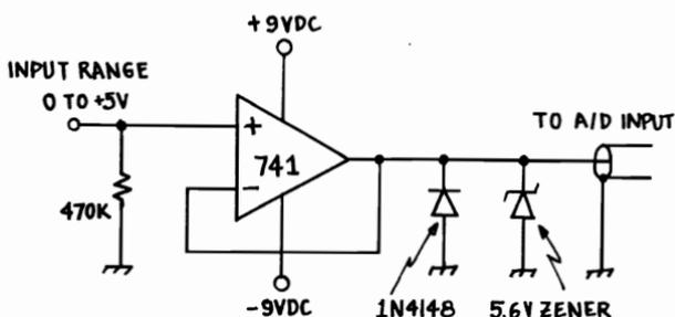
Figure 28.3 DC Buffer Amplifier
