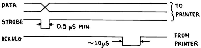
Figure 4.1 Timing Diagram of the Printer Handshake
