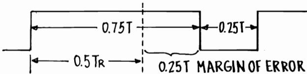
Figure 3.2 The Margin of Error for a PWM Detector that Looks at  $0.5T$ .
