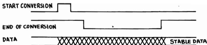
Figure 28.1 Timing Diagram of the Conversion Process
