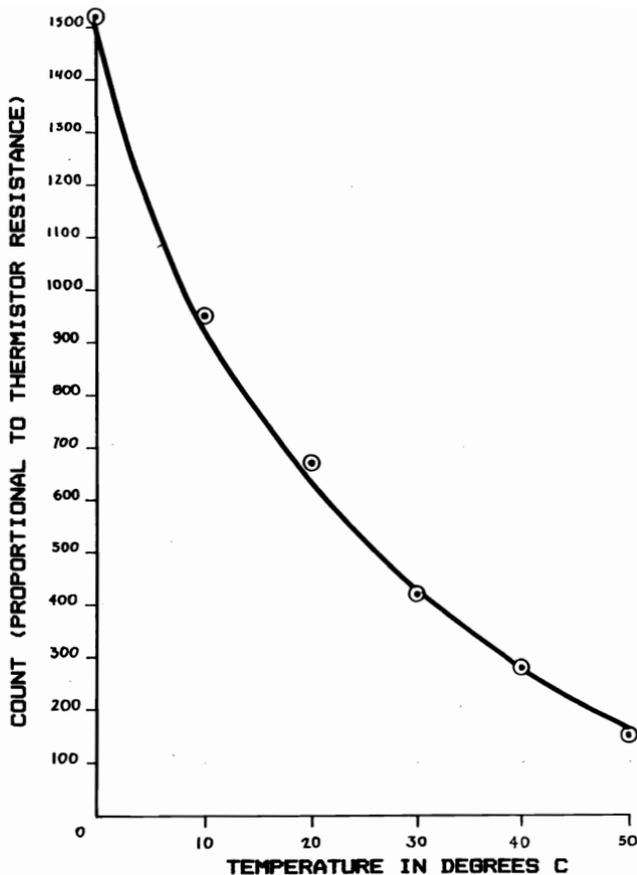
Figure 13.1 Variation of Resistance Versus Temperature for a Typical Thermistor
