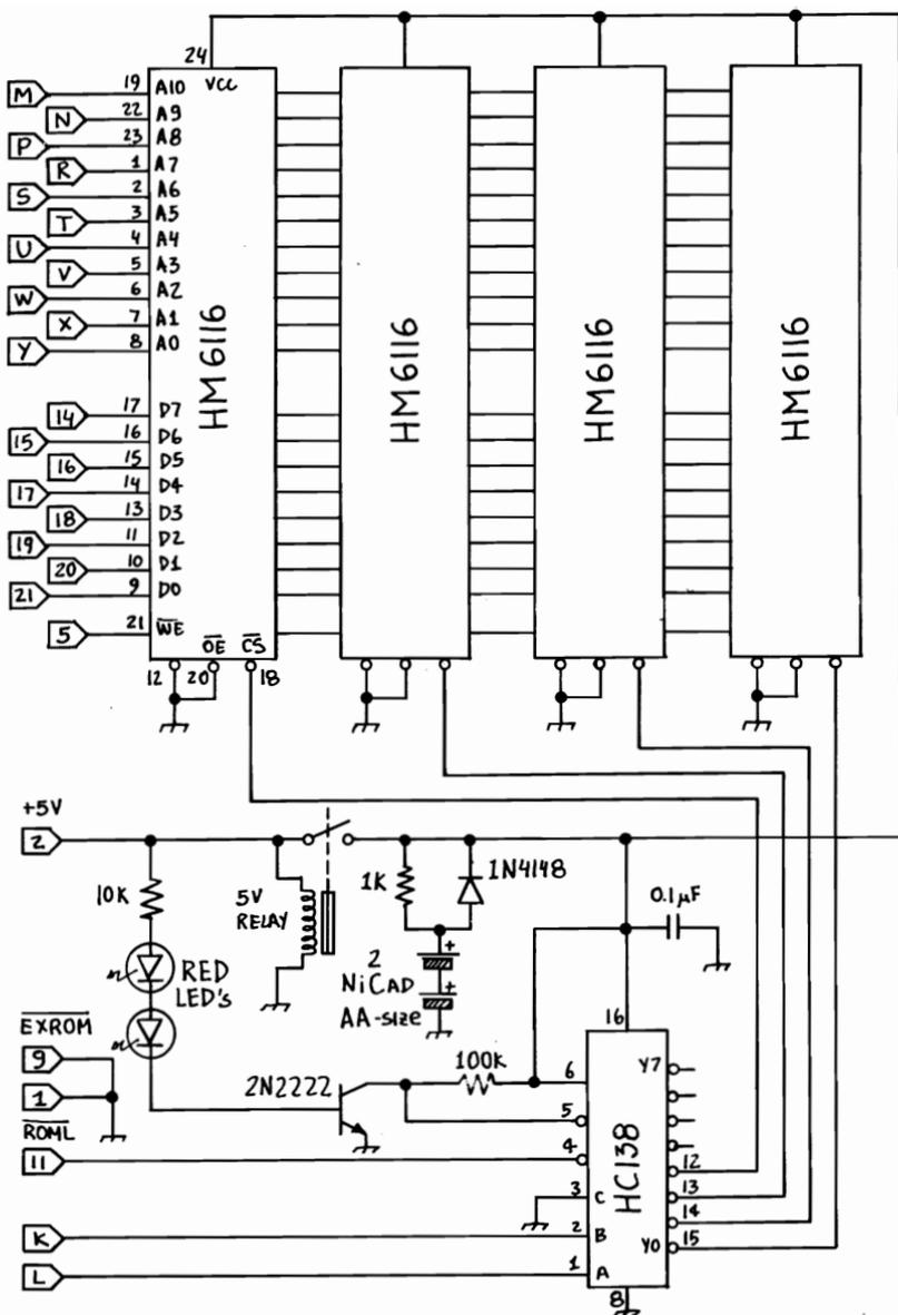
When the transistor is off, the HC138 decoder is deselected and so are the memory chips. During power down the memory IC's must not be selected because if they are, memory contents may be lost. Also, do not substitute other decoder chips for the 74HC138. It offers very low power operation required during the standby phase and at the same time is very fast so that it does not affect the operation of the 64.
