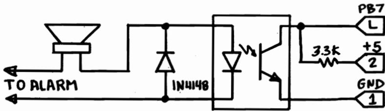
Figure 36.3 Connecting to a Smoke Alarm
