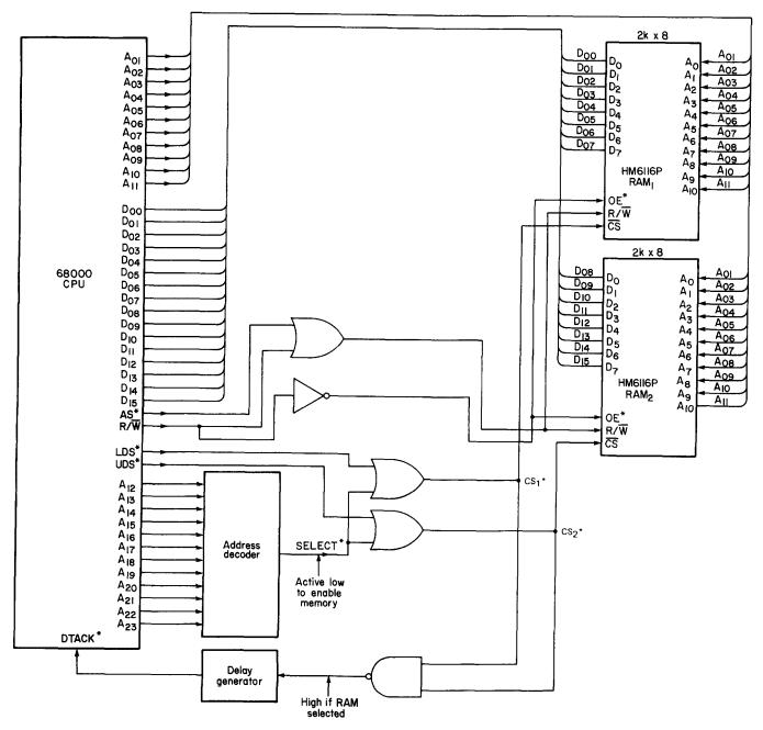
Figure 7. Connecting the HM6116P-4 RAM to a 68000 CPU
