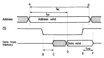
Figure 8. The timing diagram of a 68000 and HM6116P-4 combination
