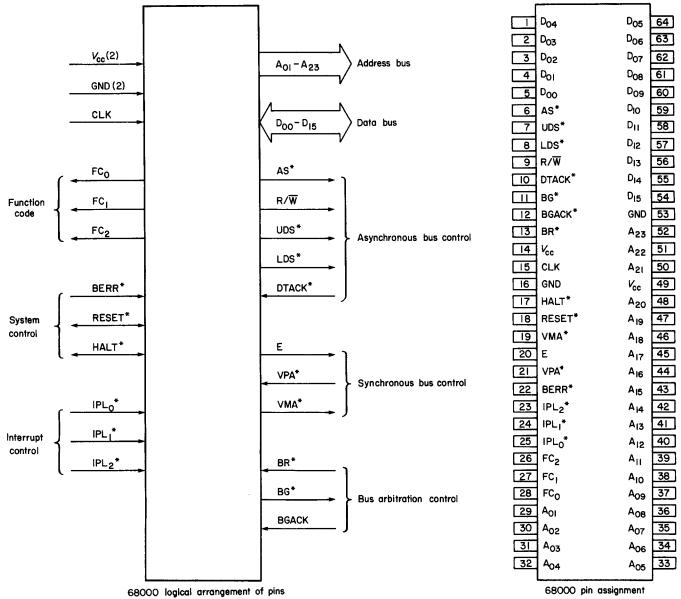
Figure 1. The pinout of the 68000
