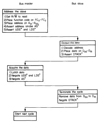
Figure 4. Protocol flowchart for a read cycle
