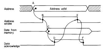
Figure 3. Asynchronous data transfer
