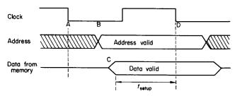
Figure 2. Synchronous data transfer
